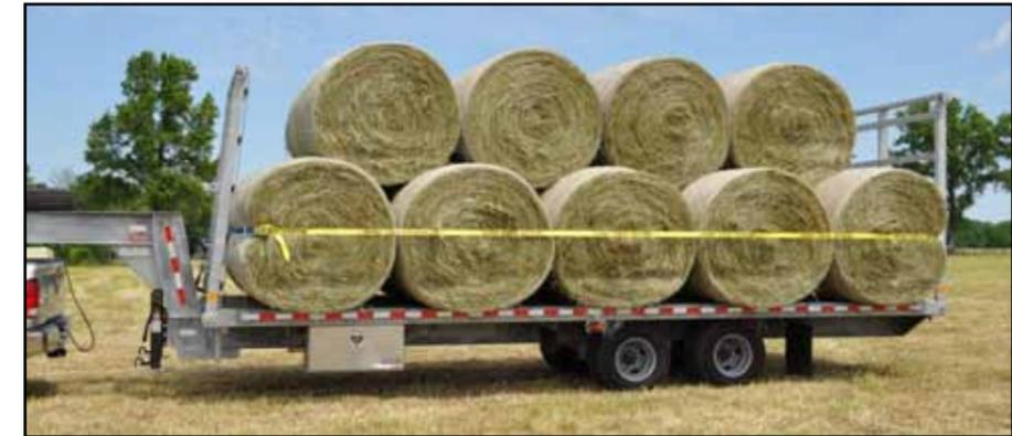
**Stake Pockets and Rub Tie Rails** are standard design across the front and rear of the trailer. This allows for easy placement of chains and straps when you need to secure a load front to rear.
